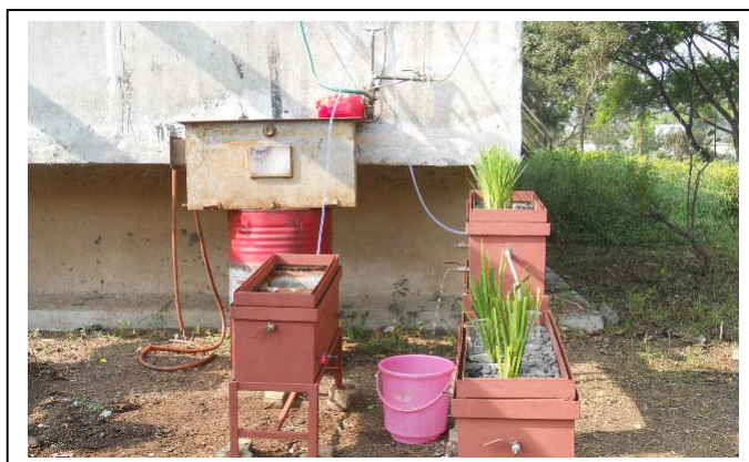
Figure 6.2 : Experimental set up of Phytorid at Tapovan
